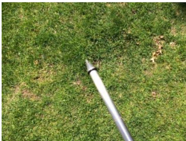
**Figure 4:** Installation of the O-ring. (Photo Credit: Steve Yergeau)
