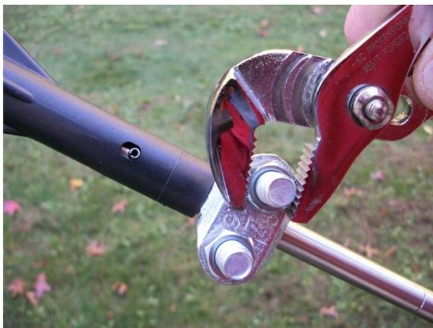
**Figure 5:** Removal of the locking ring. (Photo Credit: Steve Yergeau)
