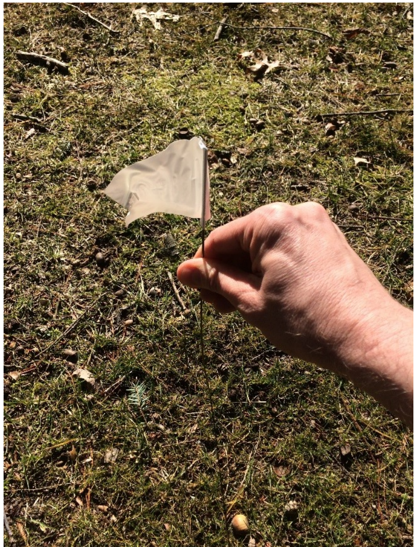
Figure 5: Wire flag being pushed into the ground to measure the soil hardness.
