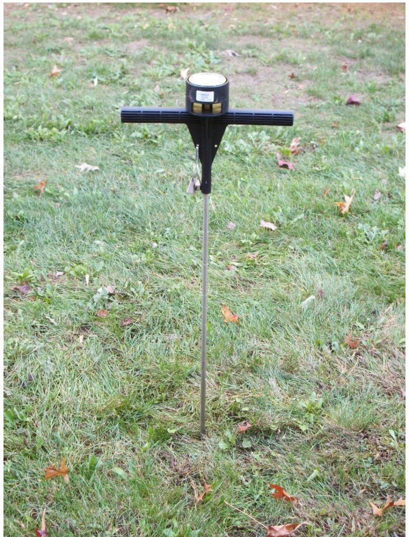
Figure 6: A static cone penetrometer, a.k.a. soil compaction tester.
